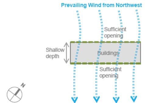
Figure 3.7 NW facing facades utilising prevailing wind
