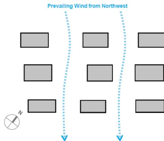
Figure 3.6 Primary roads aligned in parallel with prevailing wind direction to create wind corridors
