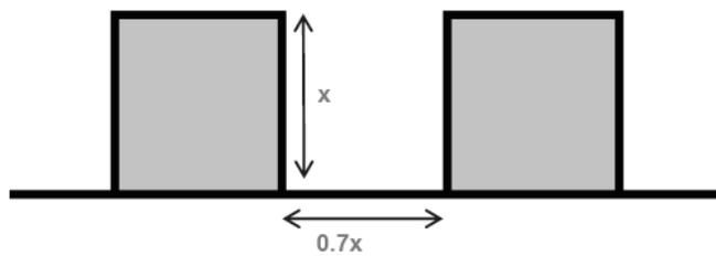
Figure 3.5 Proximities between buildings should be approximately 0.7 to 1 time of adjacent building height
