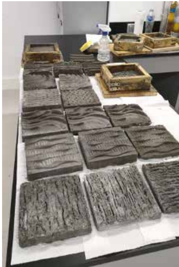
The research of adapting baroreceptive concrete in building facades (Sustainable Architecture lab)
